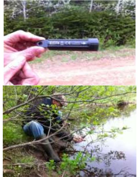
*Top: Picture of temperature logger. Bottom: SAB staff installing temperature logger in Fortune River watershed to measure water temperatures over the spring, summer and fall seasons. Photos by Becky Petersen*
